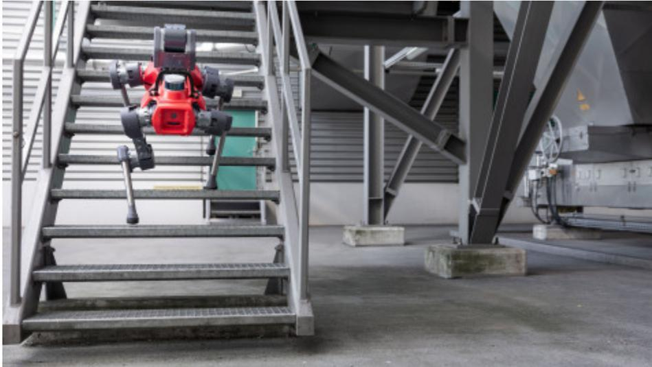
Equipped with Velodyne Lidar's Puck™ sensors, ANYbotics' four-legged robot ANYmal performs inspection and monitoring tasks in challenging industrial terrains such as mining and minerals, oil and gas, chemicals, energy and construction. (Photo: ANYbotics)
