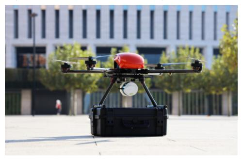
AGM Systems will utilize Velodyne's Ultra Puck lidar sensor in their new AGM-MS3 Unmanned Aerial Vehicle (UAV) mapping solution. This solution is their second generation of one of the most popular UAV lidar scanning technologies for mapping in Russia. (Photo: AGM Systems)
