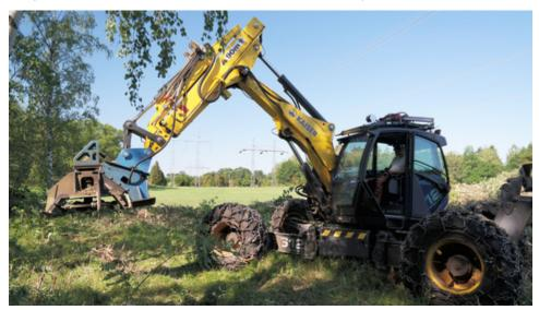
Visimind's E Cutter, a pruning machine that provides the operator efficient, precise, real-time control under power lines, using Velodyne Lidar's Ultra Puck sensor. Photo credit: Visimind Group
